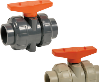
PVC - PP volle doorlaat fig 140 : PVC 1/2"-4" bsp viton O-ringen fig 142 : PVC 20-110 lijmeinden viton O-ring fig 144 : PVC 1/2"-3" bsp EPDM O-RINGEN fig 145 : PVC 20-90 lijmeinden EPDM O-ring.
